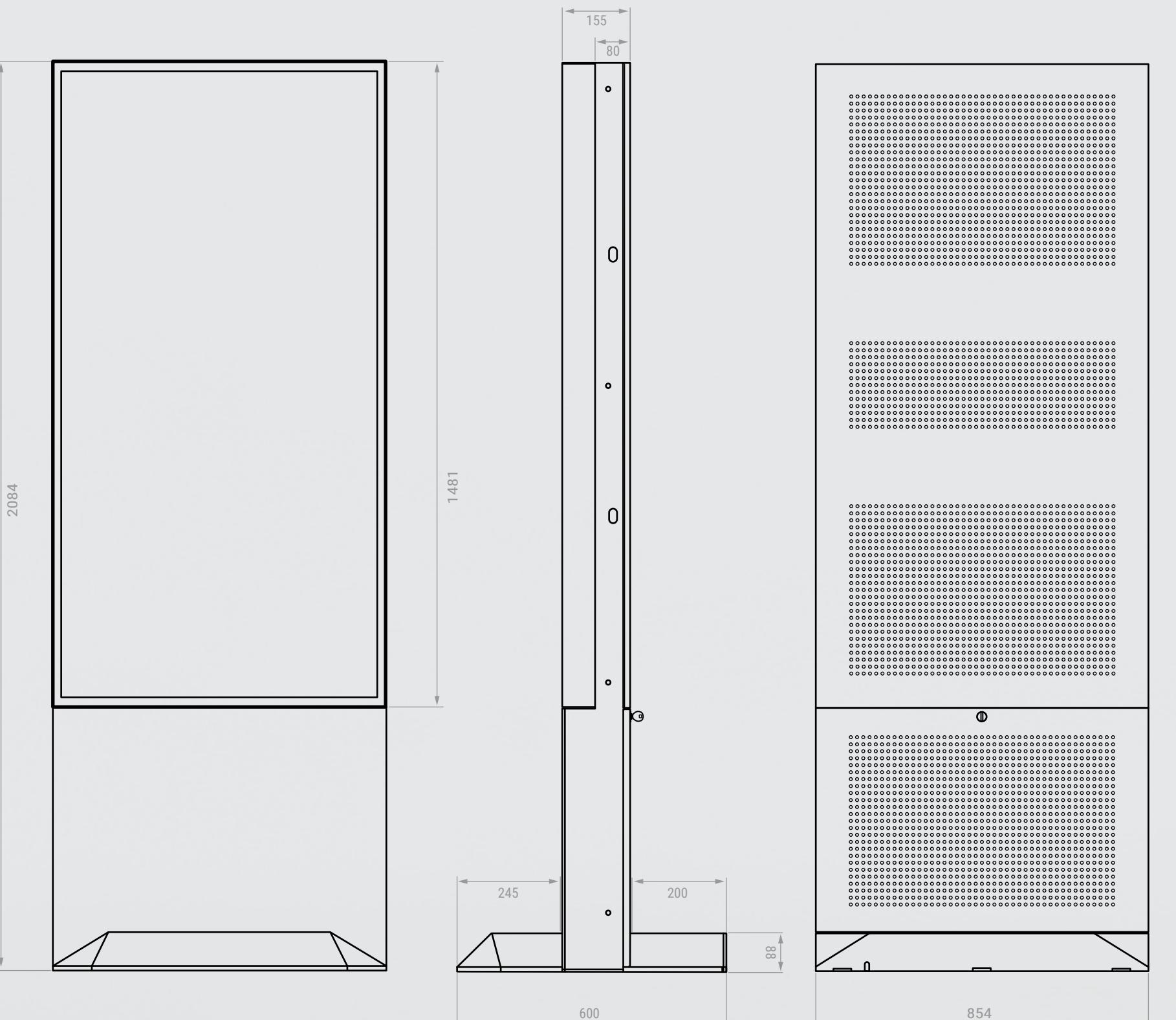
All measurements are in millimeter. Images are simulated and for illustration purposes only.
